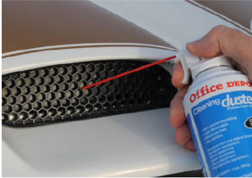
Dust Buster (or a generic “canned air” product) is commonly used to clean computer keyboards. Basically, it is cold, compressed air in a can. It works great for blasting unwanted debris from your car’s nooks and crannies. We’ve used it to blast dust from interior vents and to remove dried,
